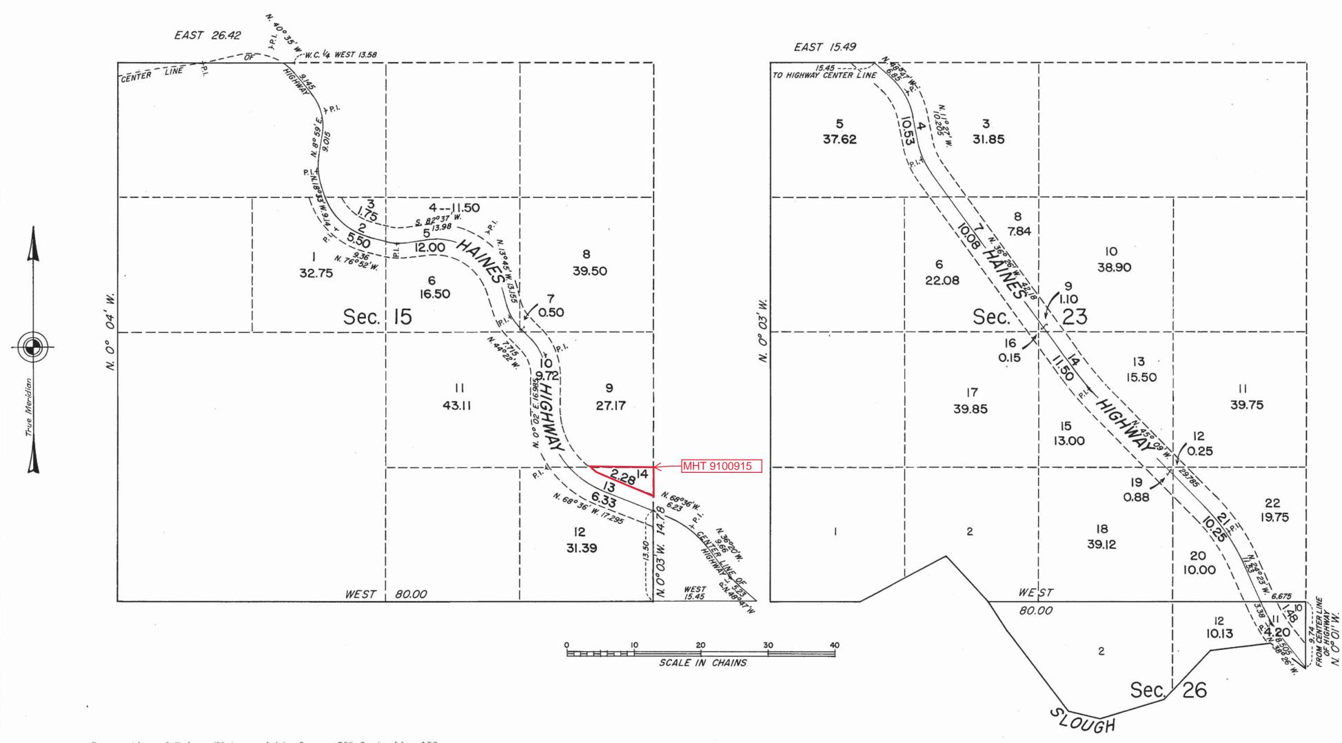
Segregation of Haines Highway right-of-way, 300 feet wide, 150 feet on each side of the surveyed center line. This survey was executed by Jack C. Means, Cadastral Engineer, September 16 to October 24, 1950, under assignment instructions dated August 11, 1950 (Group 12, Alaska).
